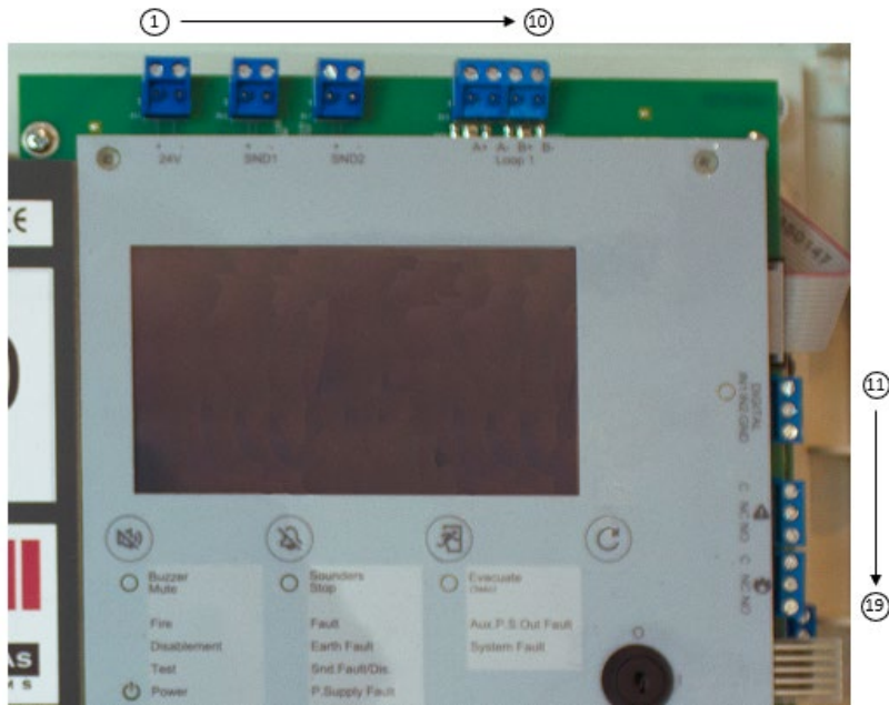
Fig. 10: Main Board connector sequence
